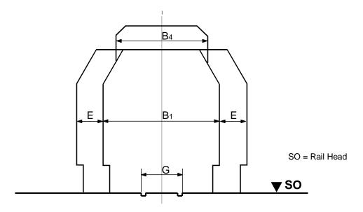
The vehicle's lateral overhang on the curve is the determining factor. Bogie equipped vehicles have the greatest overhang. The scale length of the vehicle combined with the radius of the curve determine the dimension of  $\boldsymbol{E}$ .
